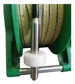
Figure 4-5 Magnetic Probe with nylon disc
