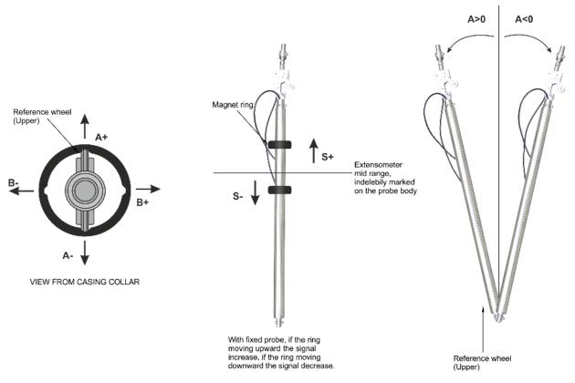
Figure 6-3 Displacement and Settlement Direction
