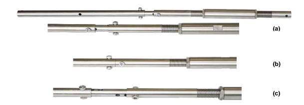
Figure 4-6 Gage coupler tubing with coarse adjustments of  $\pm 12.5$  and  $\pm 25$  mm through extension pin with six holes (left) and spacer tube and fine adjustments of  $\pm 25$  mm with chuck nut with right and left hand threads (right).
