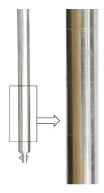
Figure 6-4 Sensor marking 100 mm for settlement measurement
