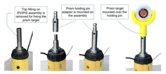
Figure 4-3 Prism target mounting accessories suitable for taking X-Y coordinates for IPIS
